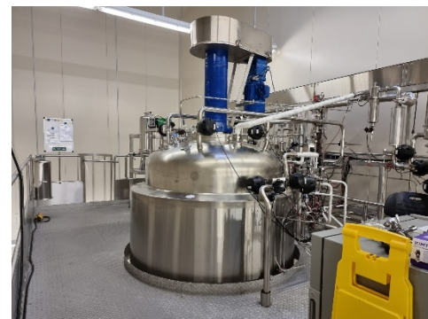
7,500 liter fermentation of Tetrahymena at CDMO side
