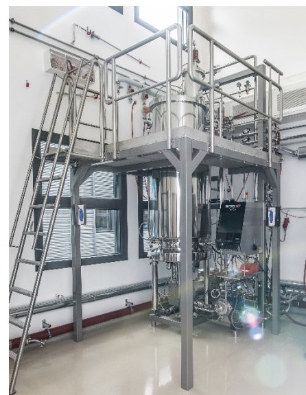
900 liter bioreactor in the labs of Cilian
