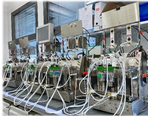
Lab scale in Münster (GER): Multi-fermenter system 12 parallel 1 L bioreactors
